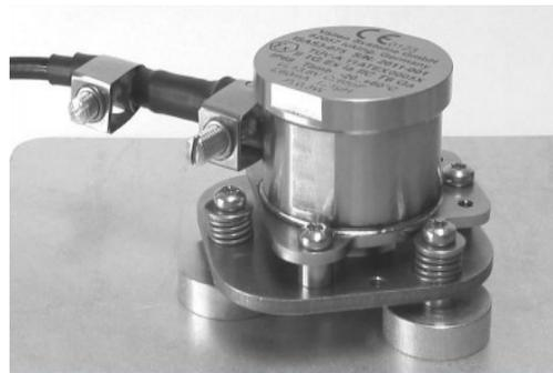
**Fig 3: Acoustic Emission Sensor**
