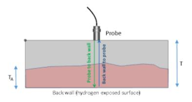
The velocity ratio measurement differentiates which between fissures and other internal It is not affected by defects. geometry, material back wall surface condition, or the measuring system.
